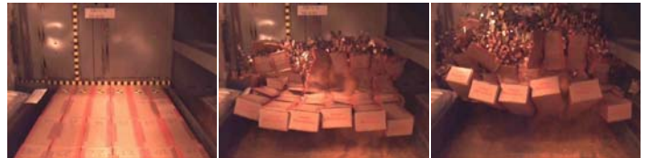
Figure 10. Sled Test Cargo Motion
