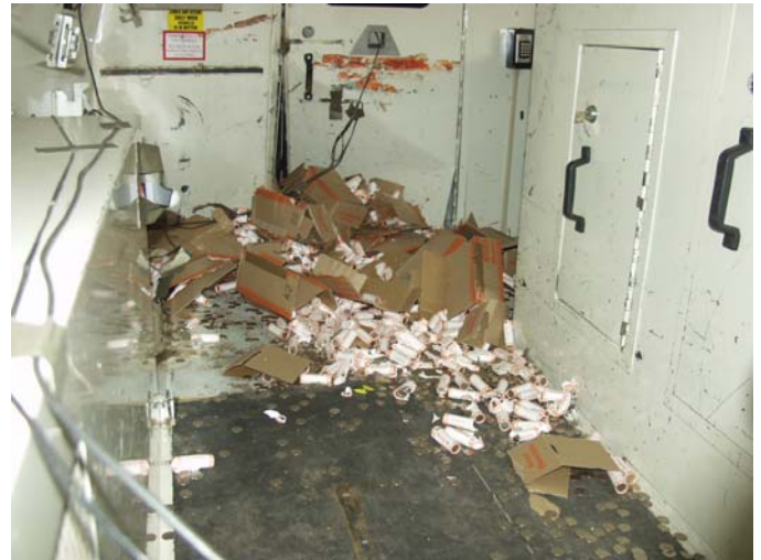
Figure 7. Post-Crash Cargo Position with Cargo Shifted Forward in Van
