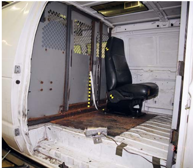
Figure 12. Post-Sled Test Cargo Barrier
